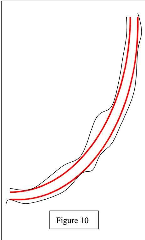
each distance value. After the corrections are applied the distance image will look as if the tool has moved perfectly along the centre of the borehole. In the case of a regular borehole it is easy to define a centre of the borehole. The problem of the correction procedure is to adapt a practical approach for the calculation of the borehole centre.
