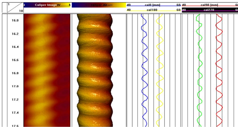
Presentation of very small (2 mm) bore hole caliper undulations induced by the drilling process
